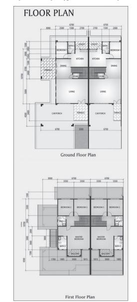
Appendix 1: Layout Plan of a Typical Double storey Terraced House
